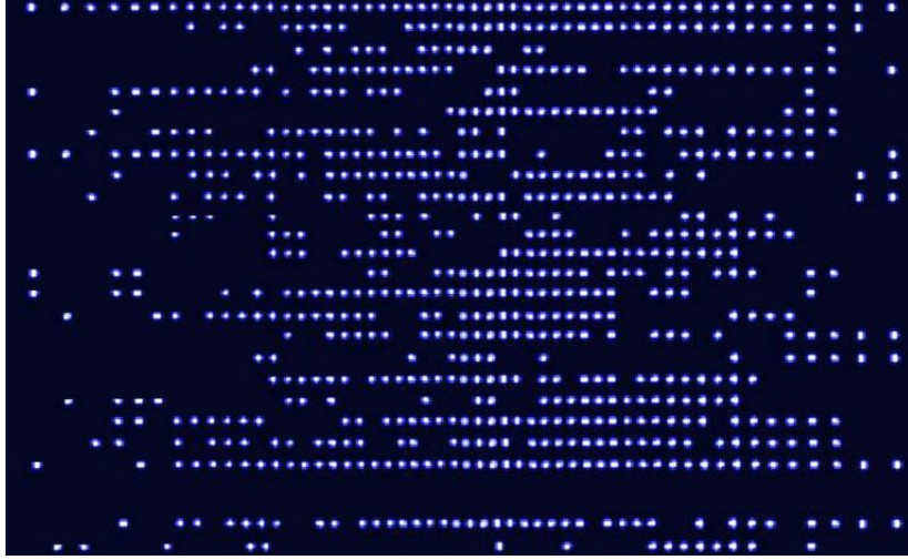
Figure 4: Trapped ion qubit readout with Dehmelt shelving. Each row corresponds to a different measurement of 53 trapped ion qubits, showing either a bright spot ( |0\rangle ) or dark spot ( |1\rangle ), in our notation. Figure from Chris Monroe's group at Maryland/IonQ. See https://iontrap.umd.edu/2017/12/01/quantum-simulation-with-individual-control-of-53-qubits/ .
